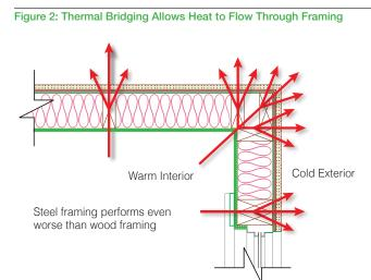
insulation provides little to no thermal benefit to framing members and other discontinuities in frame wall construction, and it is also easily compressed during installation which can further reduce insulation value as well as allow excessive airflow within the cavity. Over time, this type of insulation can also settle, sag, and absorb moisture, all of which contribute to reduced thermal performance.
