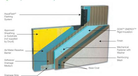
Figure 8: Dryvit's Outsulation® X System
